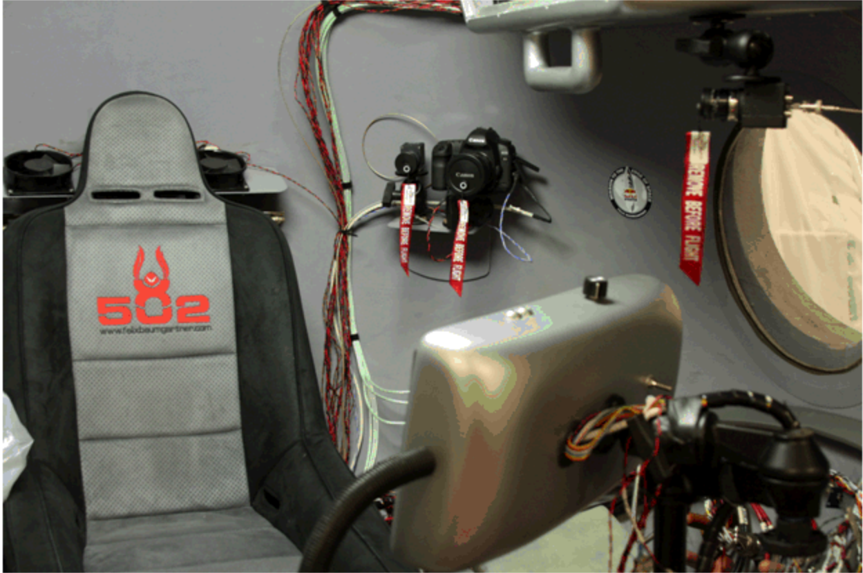
Still camera and POV camera placement inside the Red Bull Stratos capsule. @FlightLine Films
